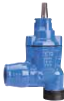
Series 11/00 Service connection angle valve with external thread on inlet and internal thread on outlet DN25-50 PN16 Ductile iron
