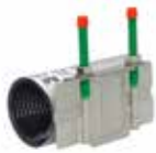
Series 748/01 Repair clamp Single band with support plate Stainless steel AISI 304 or AISI 316 NBR or EPDM rubber
