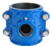
Series 10/00 Tapping saddle for uPVC and PE pipes DN50-300 Ductile iron Lower part in stainless steel from DN250
