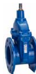
Series 06/75 Flanged gate valve Face-to-face DIN F4 Replaceable stem sealing DN50-400 PN10/16 Ductile iron
