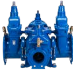
Series 18/00 Combi-cross flexible design DN100-400 PN10/16 Ductile iron With ball valves and DN100 center outlet
