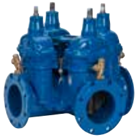
Series 18/70 Combi-cross with 4 outlets DN100-100 PN10/16 Ductile iron With ball valves and DN100 center outlet
