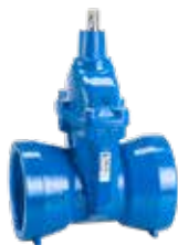
Series 33/00 Gate valve with socket ends for cast iron pipes DN80-300 PN16 Ductile iron With internal enamel
